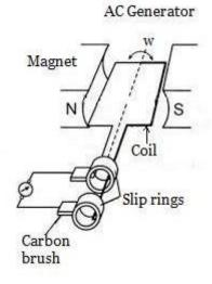
the area enclosed by the loop changes with time; this induces an emf and a current in the loop according to Faraday's law. The ends of the loop are connected to slip rings that rotate with the loop. Connections from these slip rings, which act as output terminals of the generator, to the external circuit are made by stationary brushes in contact with the slip rings.
